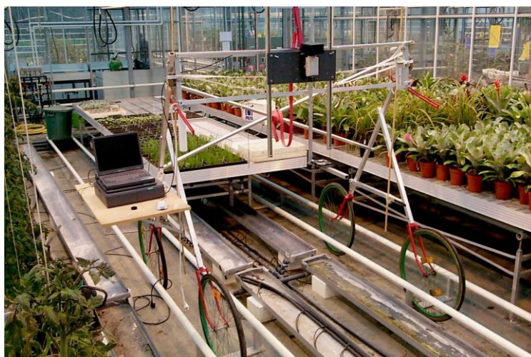
Figure 4 – Apparatus used in Leuven to carry out measurements. The “buggy” slid over the plants allowing an efficient and fast work.
