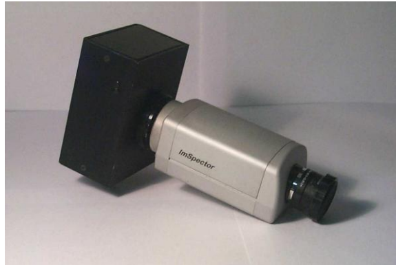
Figure 3 – ImSpector V9 spectrograph mounted on a visual monochromatic CCD camera.
